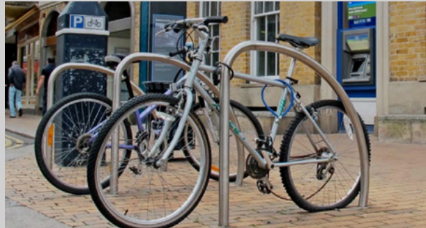
Cycle stands here are positioned to allow a clear walkway between bicycles and adjacent building edge.
